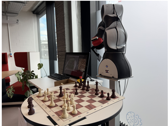
Fig. 1: Chess robot setup. SPG-based IK solver validated on a publicly available 5-DOF chess-playing robot, successfully determines correct pick poses autonomously with 100% accuracy.
