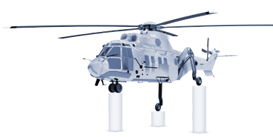
Fig. 16. Adaptive landing gear attached to the AS332 Super Puma in the preferable landing orientation
